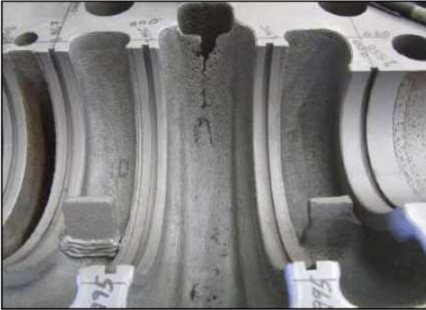
Figure 11. Pump Casing After High-P ENC
