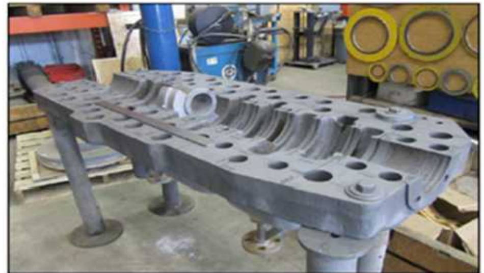
Figure 8. Cenovus Multistage Pump Casing Before ENC
