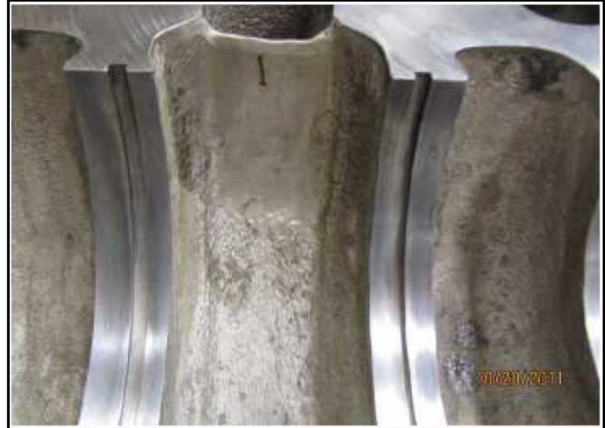
Figure 12. Steam Bypass Valve Cross Section
